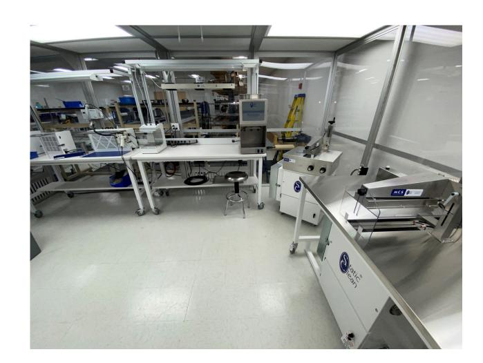
In addition to the lonstorm bars, the Fraser design introduced ionising guns that are used in a negative pressure isolator box with a separate filtered extraction system. The ionised air gun uses compressed air to neutralise and clean any particulates off the surface of the parts as they are picked for each job. These clean parts are then batched and placed into sealed containers before being delivered to the next stage of the manufacturing process.
