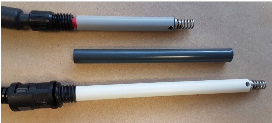
Older 30 kV Fraser connector
