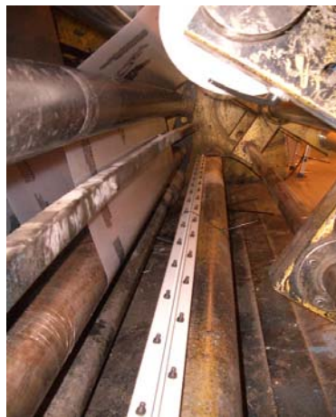
A typical winder - the bar will get dirty and must be cleaned in this type of application.
